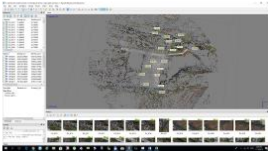
Fig. 4 – Presentation of GCP ground points
